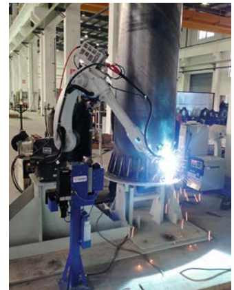
Mast robot welding for heliostats or trackers
